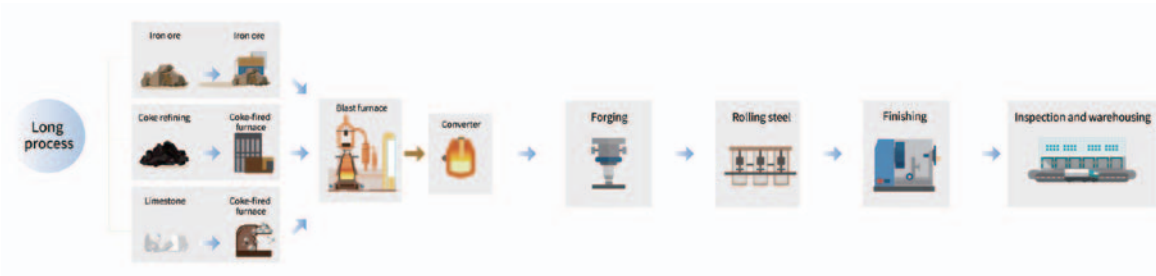
Traditional Long-Process Special Steel Manufacturing
